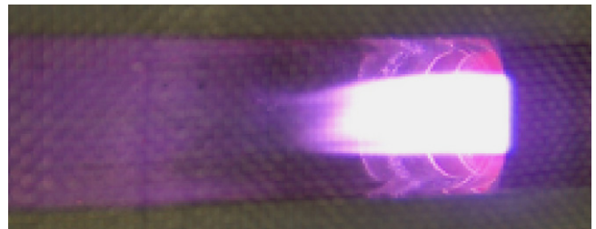
Fig. 3. Photo of the atmospheric pressure microwave discharge in methane generated by the waveguide-based nozzleless cylinder-type MPS. The methane flow rate (central flow) and the nitrogen flow rate (swirl flow) were 175 and 100\text{ l min}^{-1} , respectively. The absorbed microwave power was 4000\text{ W} .
